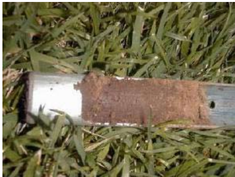
Soil probes take soil samples at depth to help determine the moisture level in the root zone. Dry topsoil but wet root zone shown may not need to be watered. Photos courtesy of Water Right.
