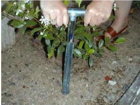
Soil probes take soil samples at depth to help determine the moisture level in the root zone. Dry topsoil but wet root zone shown may not need to be watered. Photos courtesy of Water Right.
